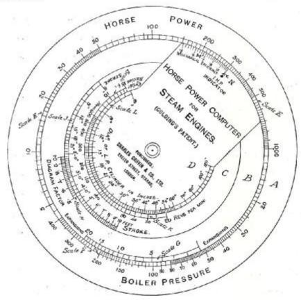
EXAMPLE II.—To find the I.H.P. of a compound engine L.P. cylinder 24-inch diameter, stroke 3 feet, revolutions 100, boiler-pressure 160 lbs., expansions 10. See illustration on this page. Set 10 on scale G to 160 on scale F.
